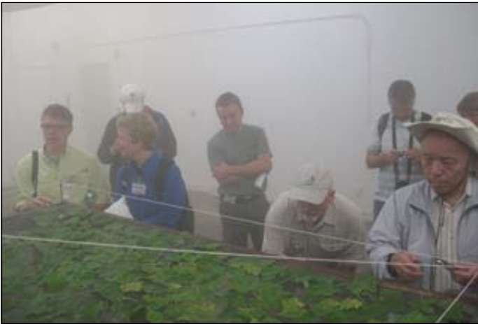
Fog chamber for white pine blister rust inoculation at Dorena Genetic Resource Center (Photo: R.Sniezko)
