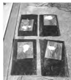
Photos 2 & 3 - Showing squirrel damage.
